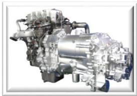
**Integrated generator-motor power system (Range Extender)**
