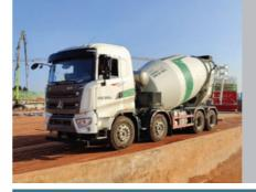
Yuchai Xin-Lan: S06-100kW P1 parallel hybrid powertrain system powered SANY hybrid concrete mixer truck
