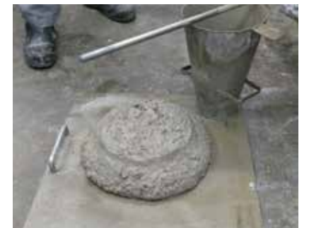
Test trials on PFAC at Island Concrete Batching Plant, Singapore
